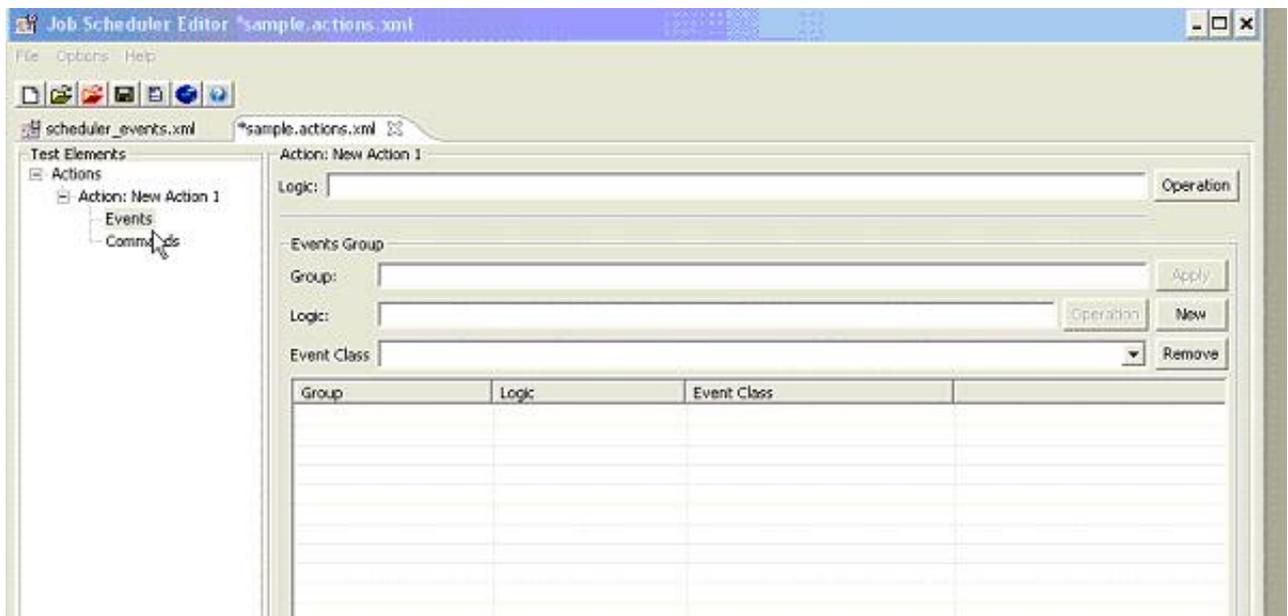
A group has a name and a logic parameter and comprises one or more events. An event class can be specified for all the events of a group. The default logic operator is OR. The logical operators possible are:
